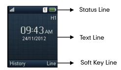
The LCD screen is divided into three parts: status line, text line and soft key line.
